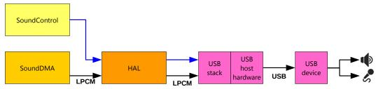
Figure 5: USB Hardware with no encoding
