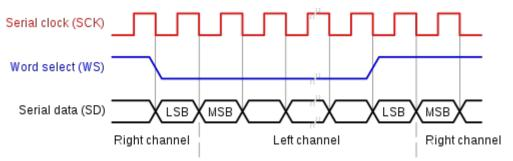
*Figure 1: I*<sup>2</sup>*S Timing Diagram (image courtesy of Wikipedia)*
