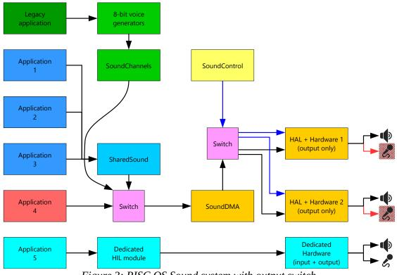
Figure 3: RISC OS Sound system with output switch
